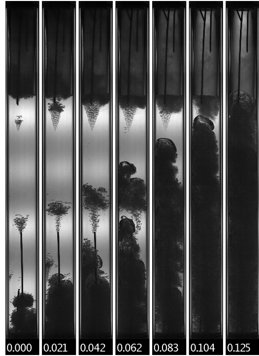
Figure 4.99: Image sequence showing “moderate” Taylor bubble formation in N_2O .
