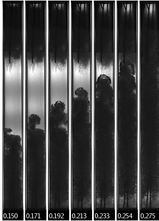
Figure 4.98: Image sequence showing “mild” Taylor bubble formation in N_2O .
