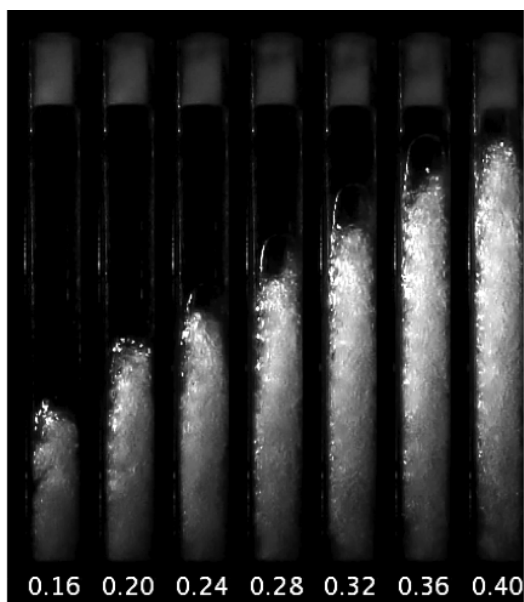
Figure 4.82: Image sequence from the high flow rate \text{CO}_2 test showing the single large bubble.
