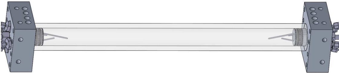
Figure 3.16: CAD model of the quartz tube with end caps. Also visible are the thermocouple probes protruding from one end cap into the tube.
