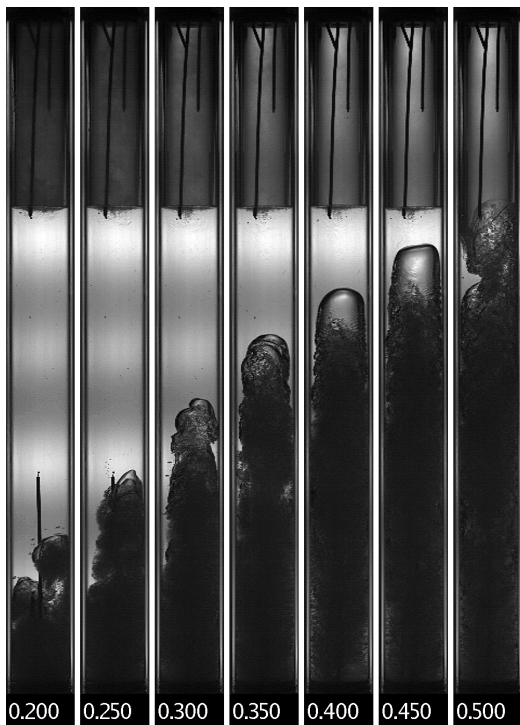
Figure 4.100: Image sequence showing “strong” Taylor bubble formation in \text{N}_2\text{O} .
