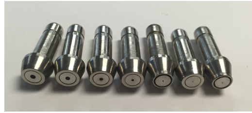
Figure 3.24: Picture of some of the orifices used in this work. The upstream side is facing the camera.
