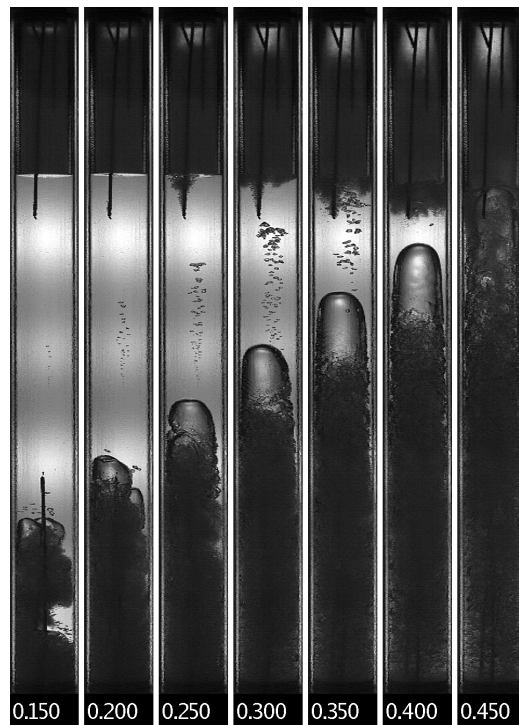
Figure 4.101: Image sequence showing “very strong” Taylor bubble formation in \text{N}_2\text{O} .
