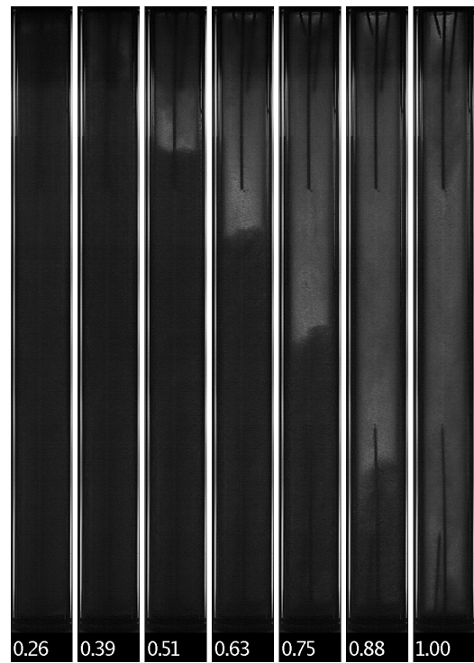
Figure 4.69: Image sequence of later times from the supercritical test. The number below each frame denotes the normalized time. Test performed with \text{CO}_2 .
