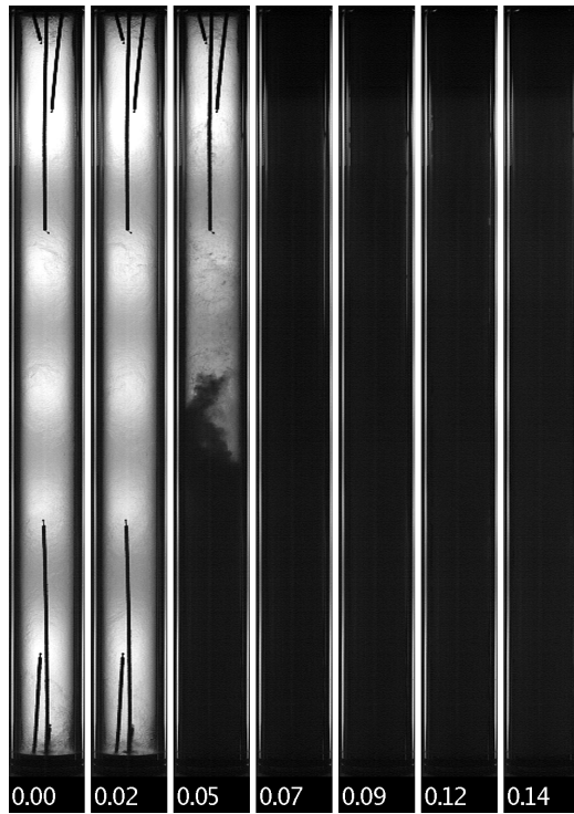
Figure 4.68: Image sequence of early times from the supercritical test. The number below each frame denotes the normalized time. Test performed with \text{CO}_2 .
