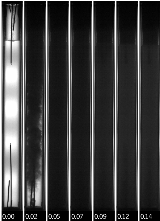
Figure 4.62: Image sequence of early times from the near critical point test. The number below each frame denotes the normalized time. Test performed with \text{CO}_2 .
