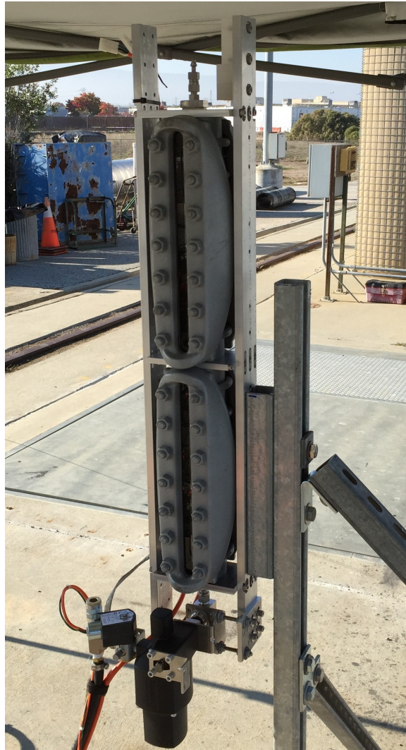
Figure 3.19: Image of the flat glass gauge. Also visible is the aluminum adapter mount and the steel strut stand.
