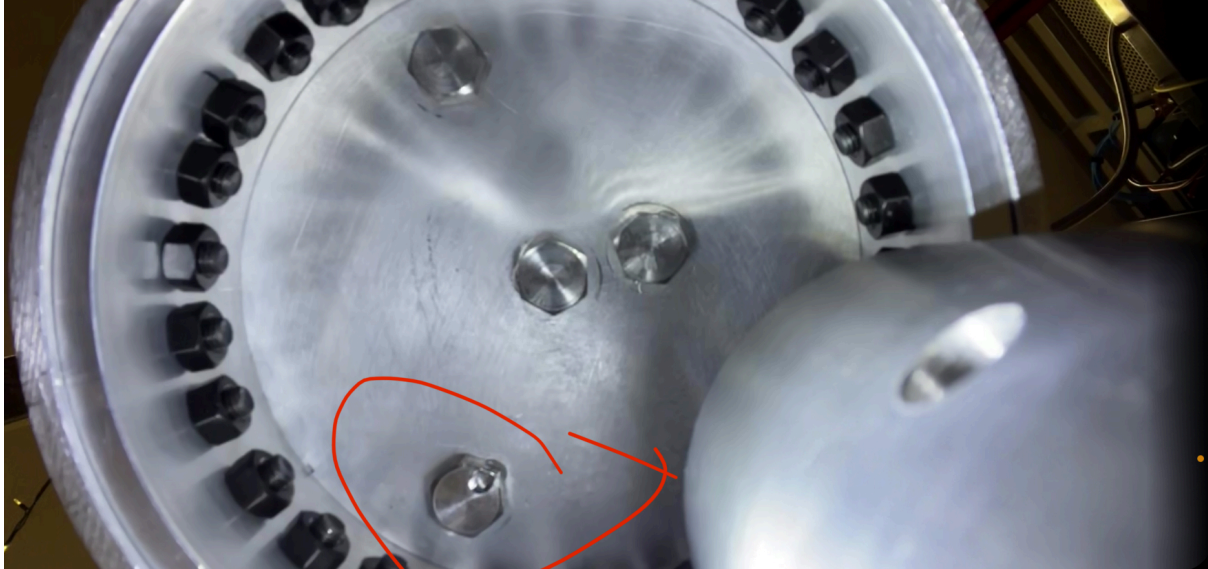
Fig. 6.2.5.2: Hydrostatic Low-pressure Leak Check on Fill Bulkhead
