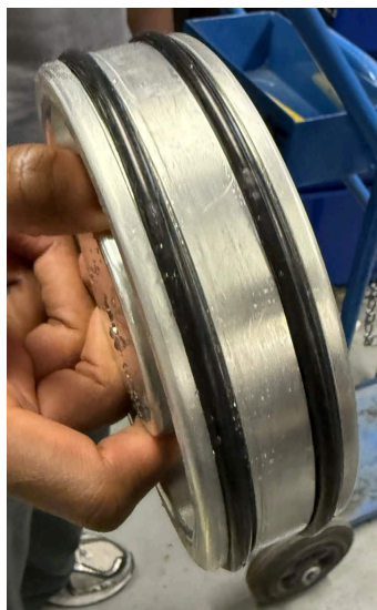
Fig. 7.2.4.1: O-rings placed on the vent bulkhead
