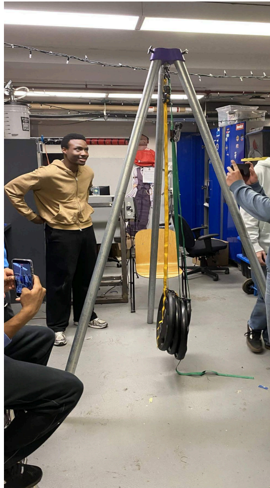
Fig. 6.3.3.2.1: Non-destructive static test of tank stand
