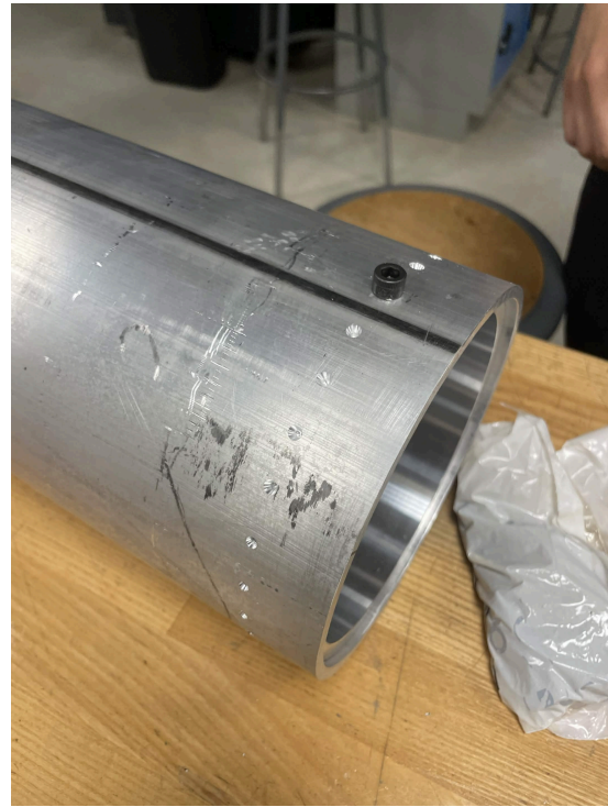
Pilot drill holes
