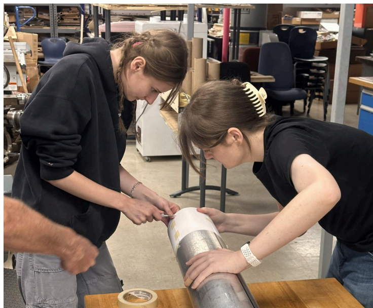
Fig. 6.2.3.2: Center punching the external tank using the drilling template.
