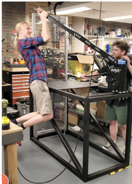
Figure A3-2: Crane undergoing structural analysis
