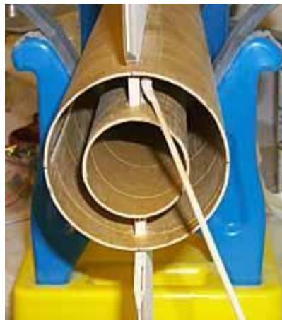
Figure 8.1 - Through-Wall Fin Mounting [ http://jrocket.com/kitbuilding.shtml ]
